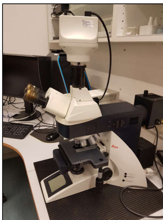
Figure 2.19 - Microscope (Leika) coupled to a Nikon DS-Ri2 camera with polarized lens used to localize plastic particles in cryosections of samples salmon's gills at the Veterinary Institute, Oslo.
